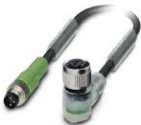
Sensor/actuator cable, 3-position, Variable cable type, Plug straight M8, on Socket angled M12 SPEEDCON, A-coded, with 2 LEDs, cable length: Free input (0.2 ... 40.0 m)
