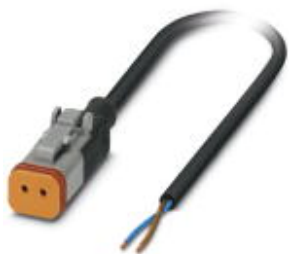
Sensor/Actuator cable, 2-position, PUR halogen-free, black-gray RAL 7021, free cable end, on Socket straight DEUTSCH DT06-2S Clip locking, with 1 LED, Cable length: 1.5 m
