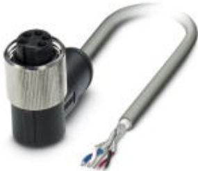
Bus system cable, DeviceNet, 5-position, PUR halogen-free, Gray RAL 7001, Free cable end, on Socket angled 7/8"-16UNF, Cable length: 10 m
