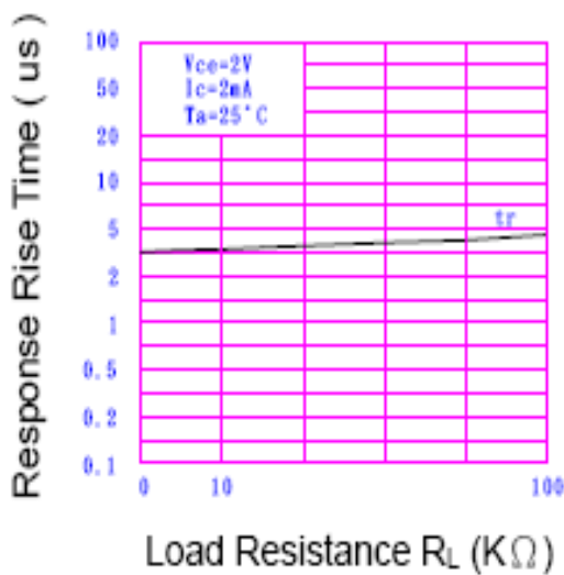
Fig.10 Response Time vs. Load Resistance
