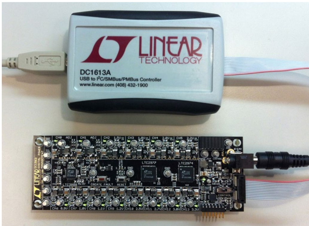
Figure 2. Connecting DC1962C Board and the DC1613 I 2 C/SMBus/PMBus Controller
