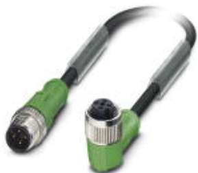
Sensor/actuator cable, 4-position, PUR halogen-free, black-gray RAL 7021, Plug straight M12, A-coded, on Socket angled M12, A-coded, cable length: 0.3 m
