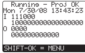
Figure 5-10 Project running, no display, and three expansion modules
