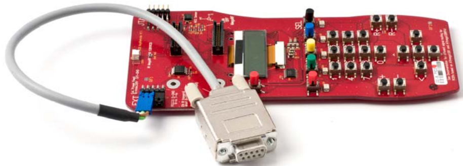
Figure 4-6. KeyRemote with RS232 cable connected.
