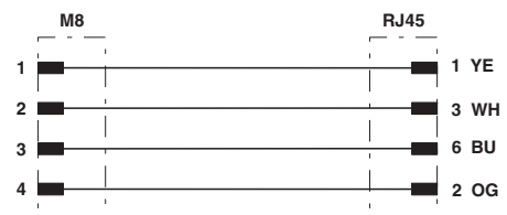
Contact assignment of the M8 and RJ45 plug
