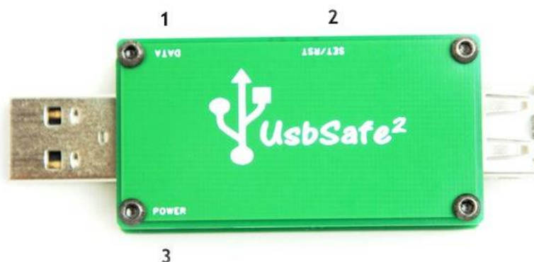
1) D2/Data LED 2) Set/Reset buttons 3) D1/Power LED
