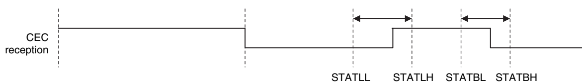
Figure 13-42. Start Bit Reception Timing
