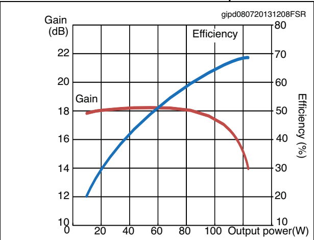
Figure 8. Gain and efficiency vs output power, freq = 945 MHz, V_{dd} = 32 V, I_{dq} = 0.4 A
