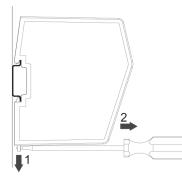
To unmount the module, a screwdriver is needed. Use the screwdriver to push the DIN-rail fastening mechanism on the back of the module down until it locks in a fixed and open position (1). Then unhook the module from the DIN-rail (2).
