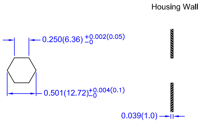
Recommended Mounting - Hole Dimensions
