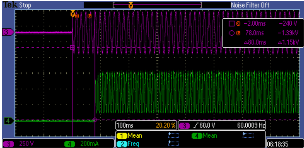
Figure 19. Start Up with AC Applied 230 V Maximum Load
