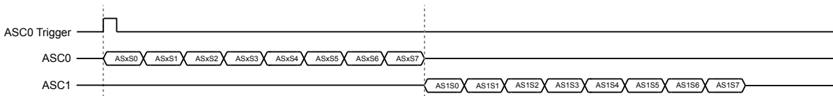
Figure 17-5. ASCx, ADCCTL.ADCMODE = 011b, 110b
