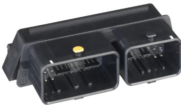
2 pocket CMC Header, series 502225 80-circuits, 32+48 Solder Tail
