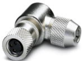
Connector, 3-position, shielded, Socket angled M8, A-coded, Solder connection, knurl material: Nickel-plated brass, external cable diameter 3.5 mm ... 5 mm
