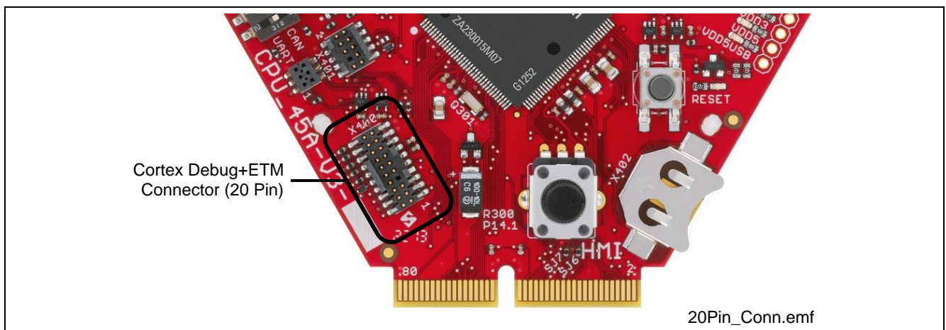
Figure 14 Cortex Debug+ETM Connector (20-pin) Layout
