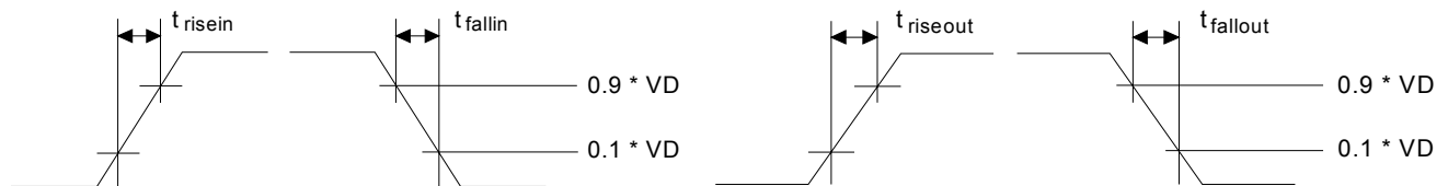
Figure 1. Rise and Fall Times
