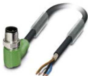
Sensor/actuator cable, 4-position, Variable cable type, shielded, Plug angled M12 SPEEDCON, A-coded, on free cable end, cable length: Free input (0.2 ... 40.0 m)
