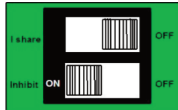
DIP Switch for Current Share & Inhibit/Enable for powerMods XgG to XgL and Xg1 to Xg5
