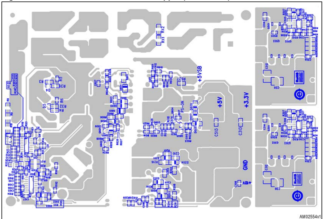
Figure 39. Bottom side silk screen and copper (mirror view)
