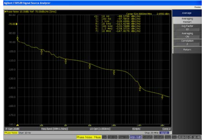
Fig 79. LO Phase Noise vs. Frequency Offset, LO = 525 MHz, RMS Phase Error Integrated from 2 kHz to 18 MHz, PLL Loop Bandwidth = 300 kHz
