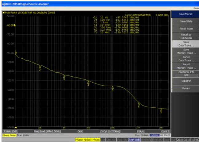
Fig 78. LO Phase Noise vs. Frequency Offset, LO = 300 MHz, RMS Phase Error Integrated from 2 kHz to 18 MHz, PLL Loop Bandwidth = 300 kHz
