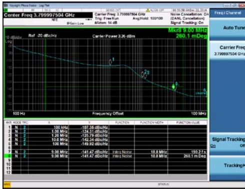
Figure 206. LO Phase Noise vs. Frequency Offset, LO = 3800 MHz, RMS Phase Error Integrated from 2 kHz to 18 MHz, PLL Loop Bandwidth = 300 kHz, Spectrum Analyzer Limits Far Out Noise
