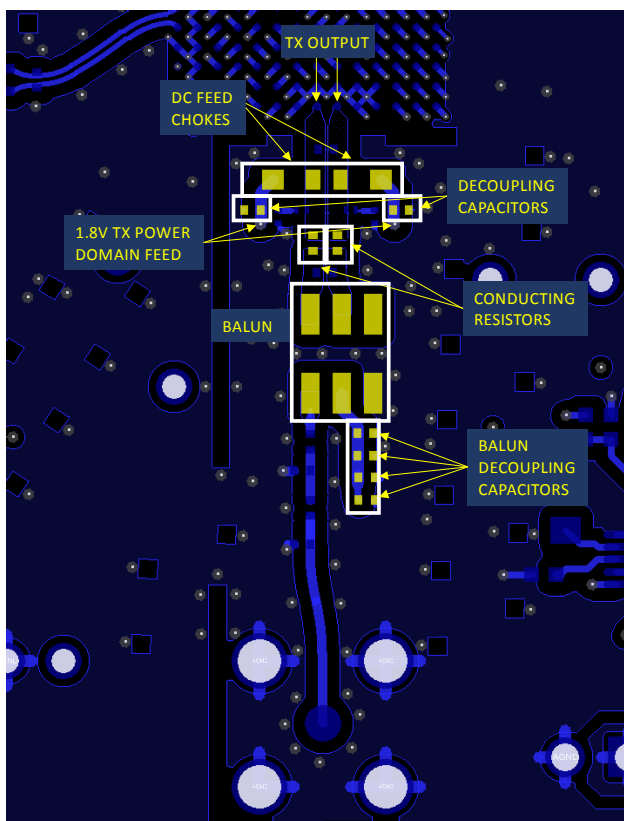
Figure 283. The Transmitter DC Chokes and Balun Feed Supply
