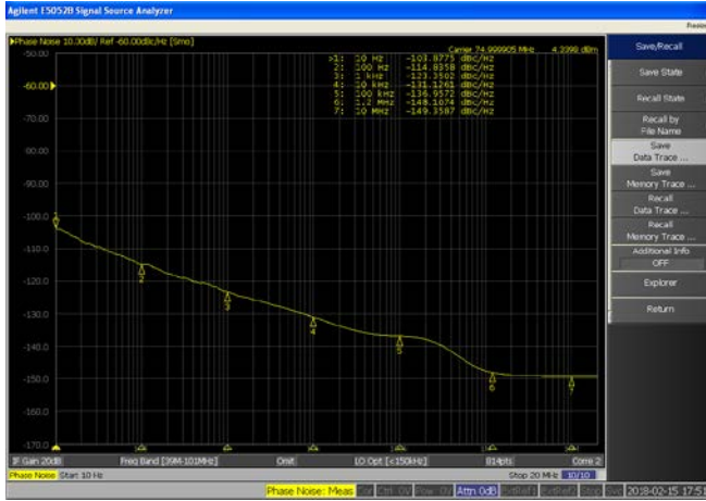
Fig 77. LO Phase Noise vs. Frequency Offset, LO = 75 MHz, RMS Phase Error Integrated from 2 kHz to 18 MHz, PLL Loop Bandwidth = 300 kHz
