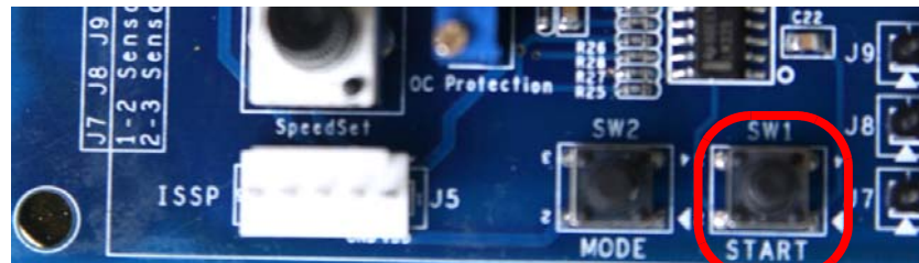
Figure 6 Press Start Button to Start the Motor
