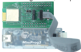
Fig 3: Programming/Debugging with MiniProg3
