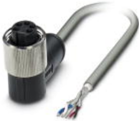
Bus system cable, DeviceNet, 5-position, PUR halogen-free, Gray RAL 7001, Free cable end, on Socket angled 7/8"-16UNF, Cable length: 2 m
