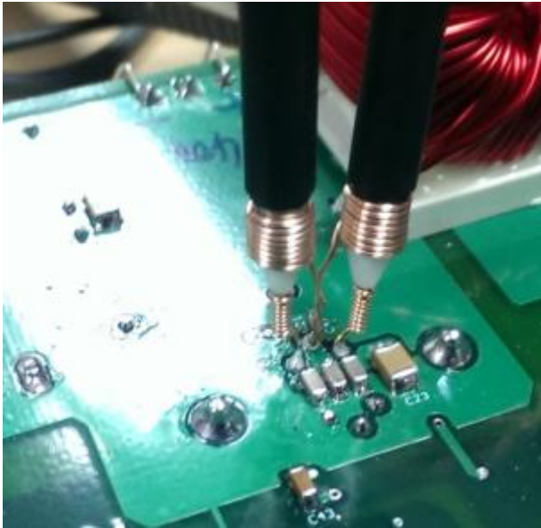
Figure 8. Low-inductance probing of fast, high-voltage signals
